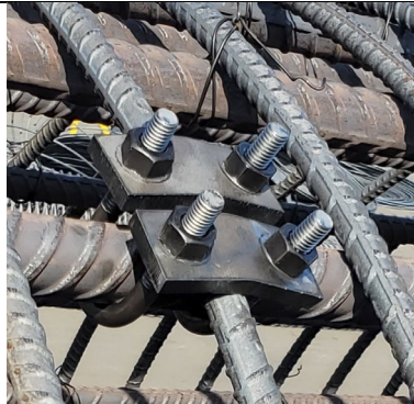
Bending of the U-bolt connector plates in a tight-fit connection
